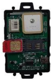
Unlock the card holder and put in an available SIM card like this
